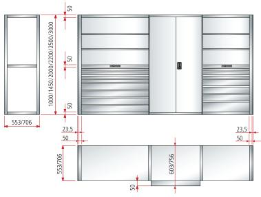
**G** = Unit length (without side panels) Unit length (with side panels) = sum of installed widths + sum of side frames = sum of installed widths + sum of side frames + 47 mm
